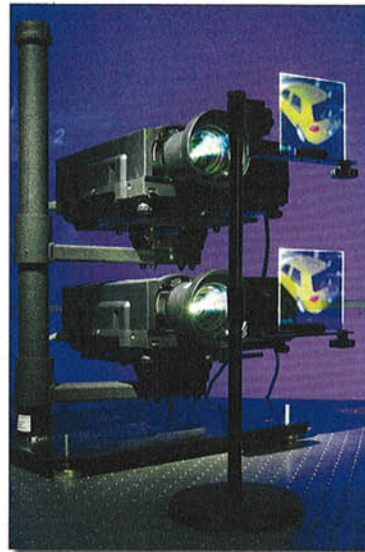
Dual projectors provide the appropriate polarization imagery for each eye with this approach from ColorLink.
