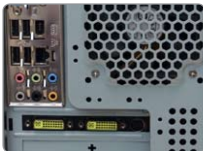
Front image of back panel, Graphics card shown at the bottom ( For the specification of our monitor, graphics card must be compatible with "Dual output" )
